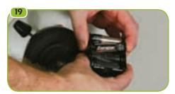
Place 8-AA batteries (user supplied) inside the battery holder.
